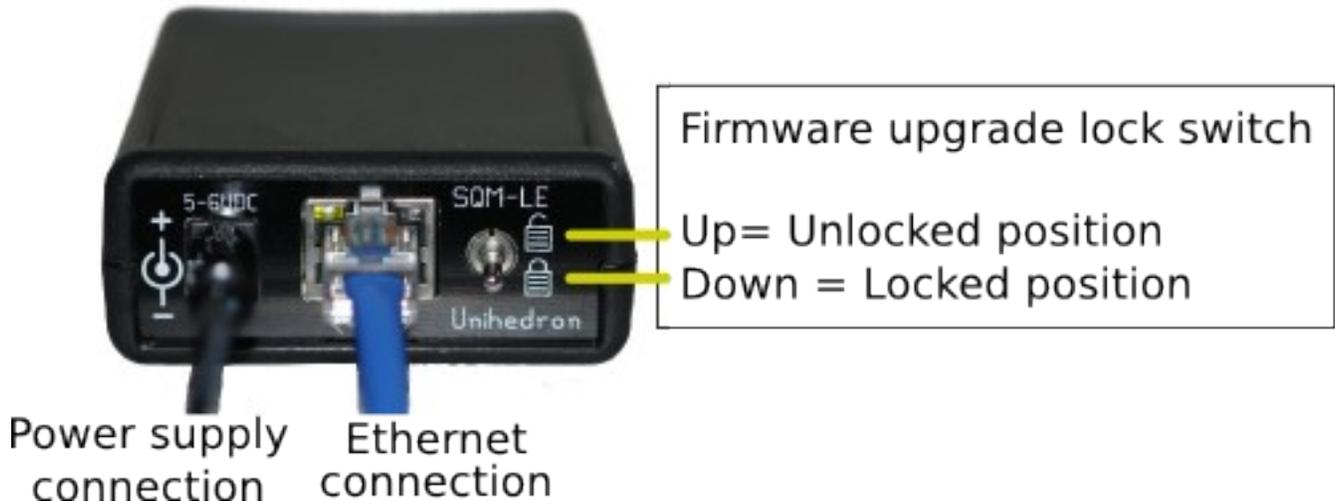
Power supply connection    Ethernet connection
