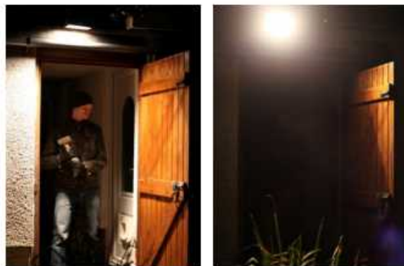
Light angled correctly Light angled incorrectly
